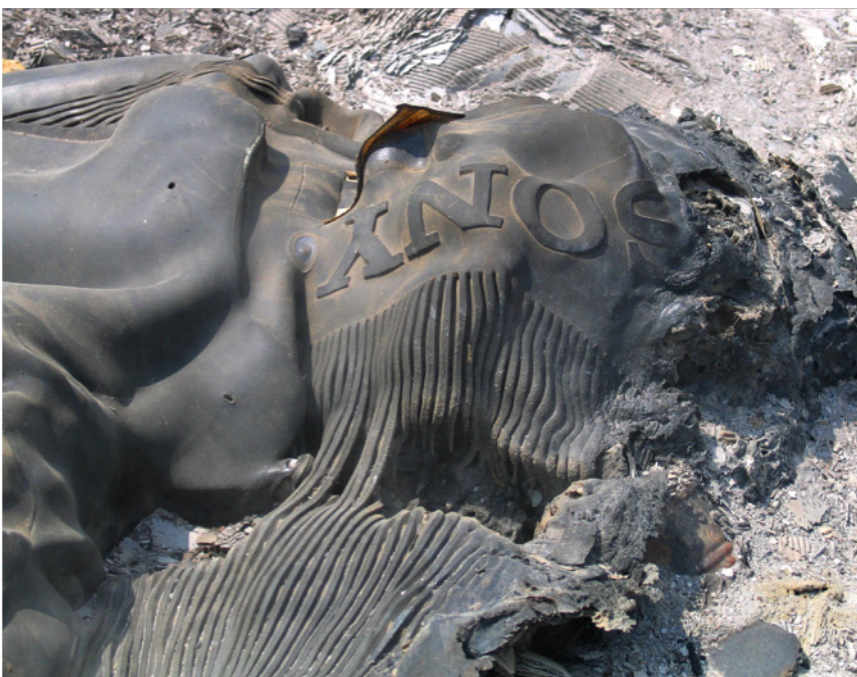
Figure A4: Melted imported CRT from the routine burning of e-waste behind the Alaba market in Lagos, Nigeria. ©BAN 2005.
