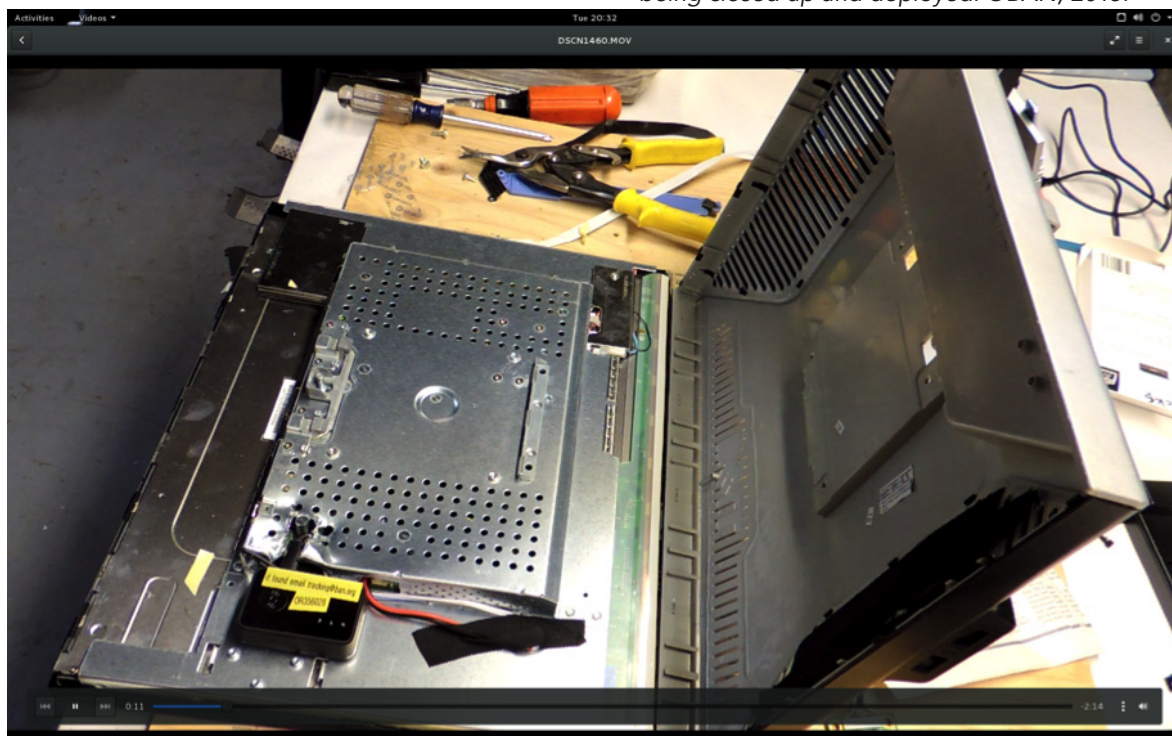
Figure A22. Screen shot of typical installation video, shot for each deployment. Shown here is a tracker being installed inside an LCD before being closed up and deployed. ©BAN, 2015.
