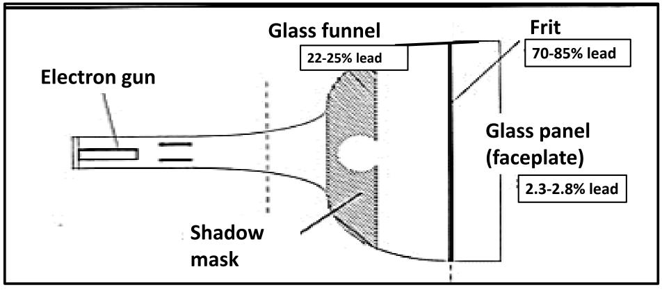
Cathode ray tubes typically contain about 4 pounds of lead, mostly located in the glass funnel and frit, and generally test as hazardous waste under U.S. regulations.
