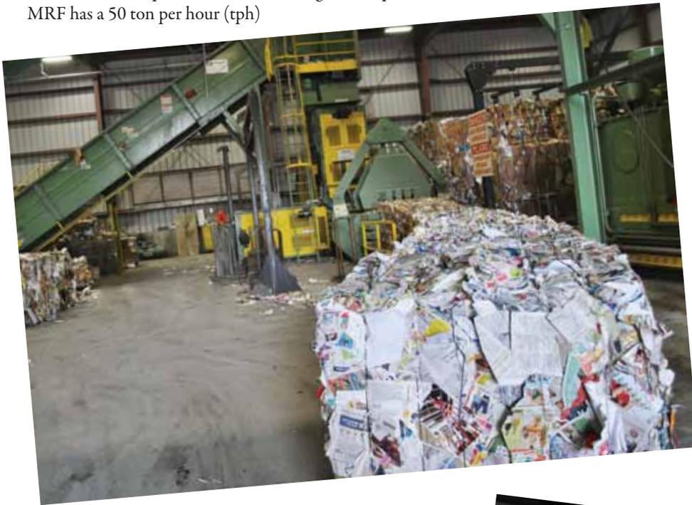
capacity, much greater than the previous system's capacity of 30 tph for fiber and 20 tph for mixed containers.
